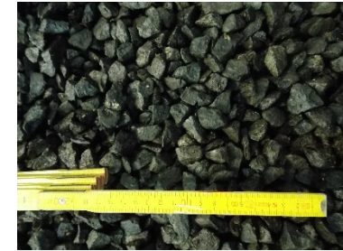
Filter layer (50-100 g) Harbour side armour
