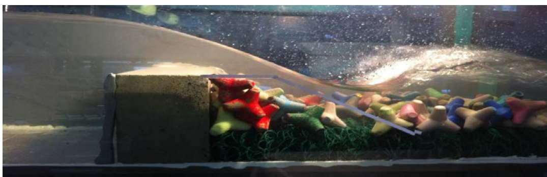
Fig.3.10. Overtopping of a composite breakwater by outgoing tsunami wave (note the heavy damage) Adapted from: (Esteban, Miguel, et al., 2013)
