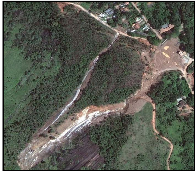
Figure 3: Debris slide burying houses and blocking a road as seen in Geoeye-1 imagery recorded shortly after a major landslide event in Brazil, January 2011. Source: GoogleEarth
