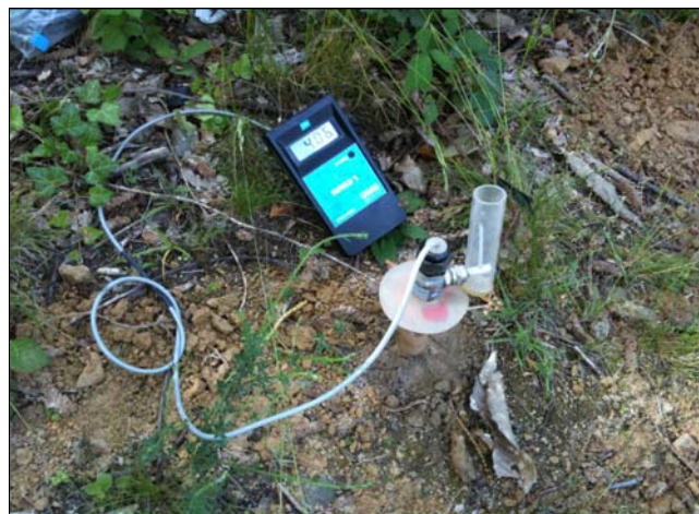
Figure 56: Tensiometer setup for matric suction measurements.
