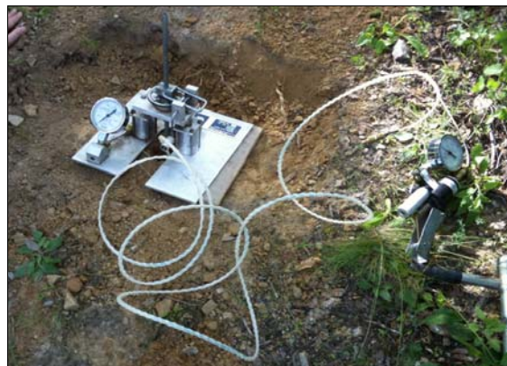
Figure 54: BST in situ measurements setup.
