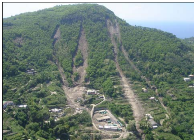
Figure 32: Monte Vezzi landslides triggered by a heavy rainstorm in the morning of April 30, 2006.
