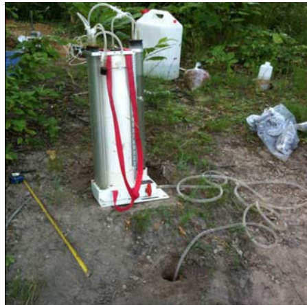
Figure 55: Amoozometer measurements setup.
