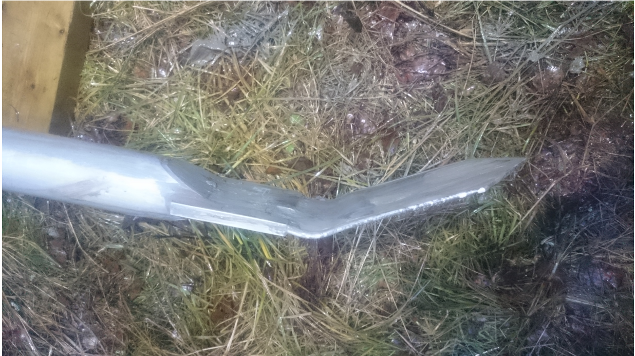
Figure 3.2: Damaged earth pressure cell after first trial installation.
